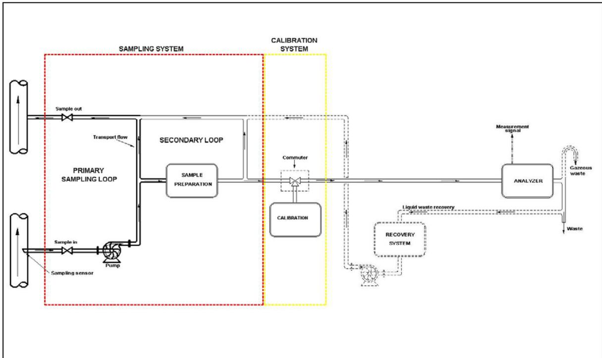
**FIGURE 1. CONTINUOUS ANALYSIS SYSTEM**
