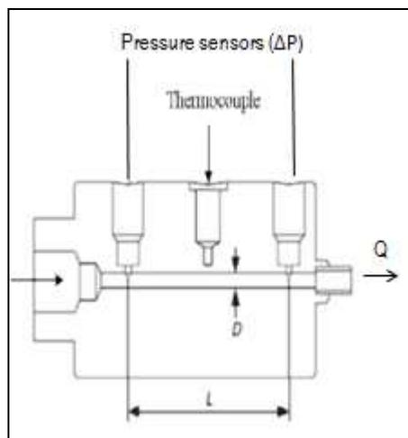
**FIGURE 1. SCHEMATIC PRINCIPLE OF THE CAPILLARY SENSOR**
