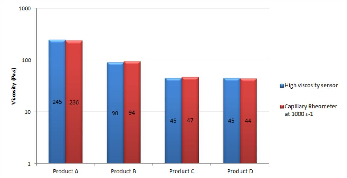
**FIGURE 16. COMPARATIVE RESULTS WITH IN-LINE VISCOMETER AND OFFLINE CAPILLARY RHEOMETER**
