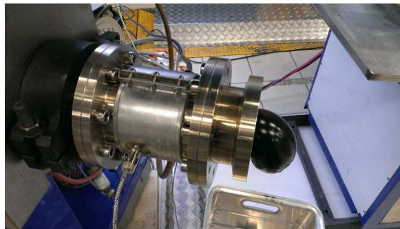
**FIGURE 13. VISCOSITY SENSOR AND CONNECTING PIECE INSTALLATION ON EXTRUDER**
