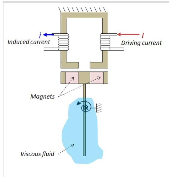
**FIGURE 2. PRINCIPLE OF THE VIBRATING VISCOSITY SENSOR AT RESONANCE FREQUENCY**
