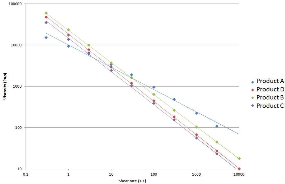
**FIGURE 15. PRODUCTS A, B, C AND D VISCOSITY VS SHEAR RATE ON LABORATORY RHEOMETER**
