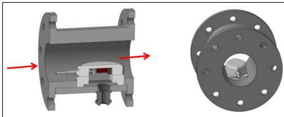
**FIGURE 7. NEW VISCOSITY SENSOR FOR EXTRUDER**
