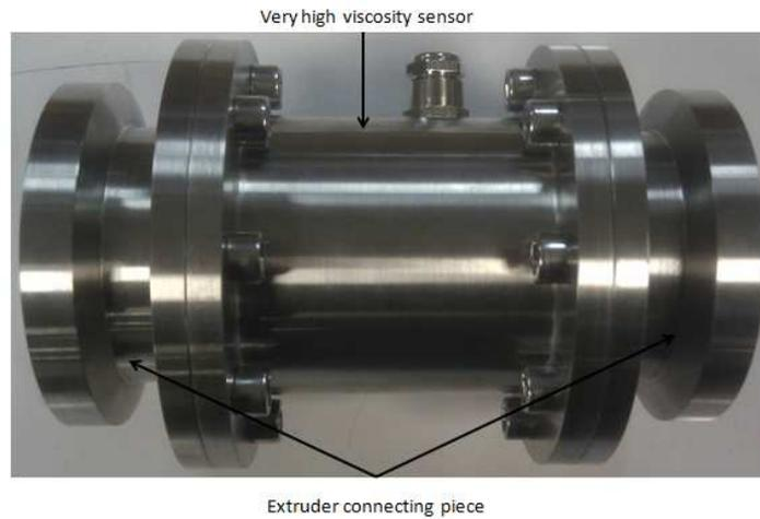
**FIGURE 8. NEW VISCOSITY SENSOR FOR EXTRUDER WITH CONNECTING PIECE**
