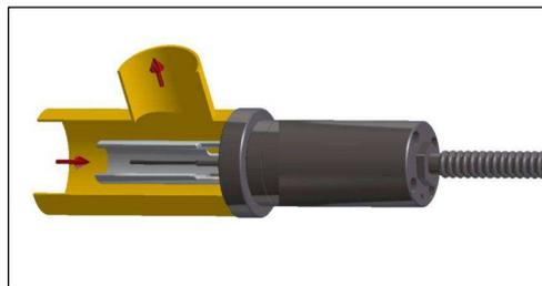
**FIGURE 4. USUAL PIPE ANGLE MOUNTING FOR VISCOSITY SENSOR**
