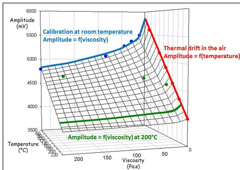
FIGURE 10. 3D FIT WITH CURRENT DRIVE
