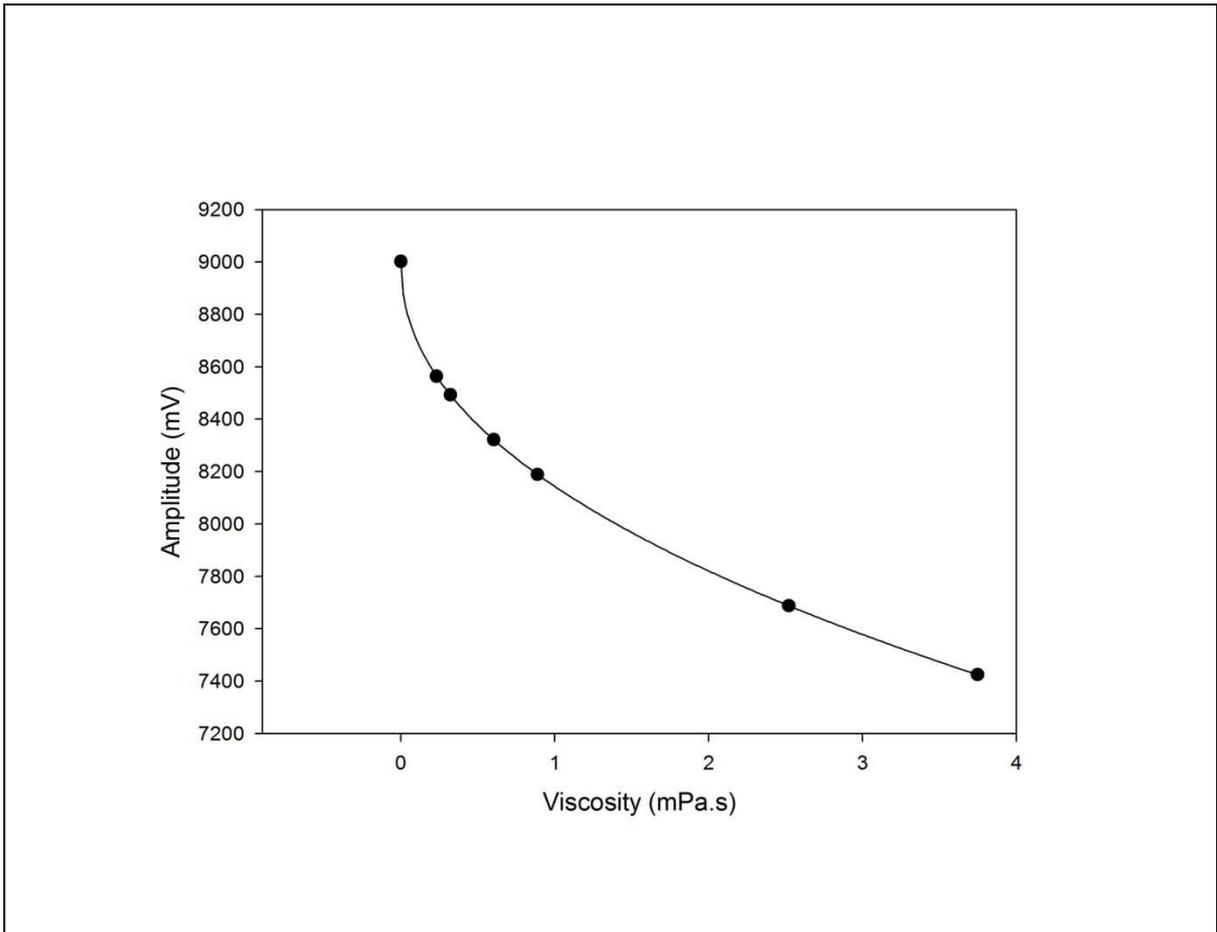
**FIGURE 4. VISCOSITY CORRELATION RESULTS ON CERTIFIED MINERAL OIL**
