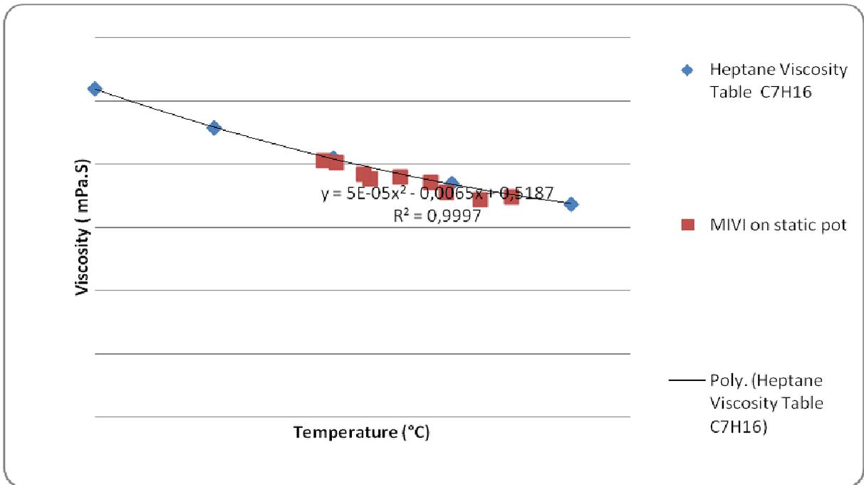
**FIGURE 5. MEASUREMENT TEST WITH HEPTANE**
